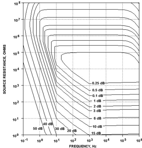
Figure A-1, Model 5184 Noise Figure Contours (Typical)
