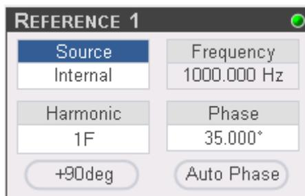
drives a phase locked loop which in turn drives the reference channel. When the instrument is set to internal reference mode, the internal precision quartz stabilized oscillator is used to generate the sinewave output at the OSC OUT connector.
