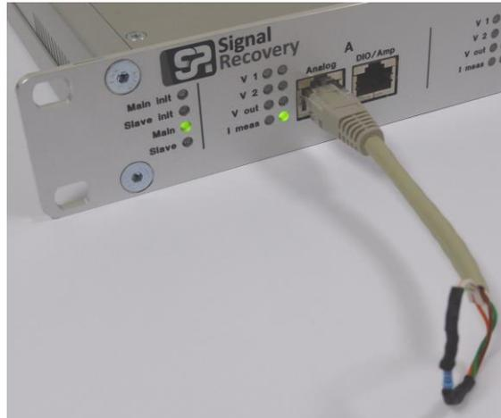
Figure 7, Model 9120 Test Fixture Connected to Module A Analog Input
