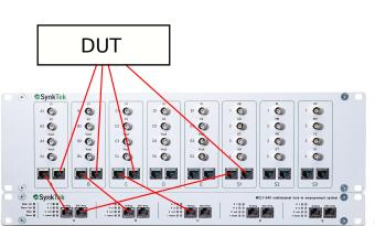
The BB8-BNC is inserted between the cryostat and the device under test. Different signals can be accessed by BNC connectors.
